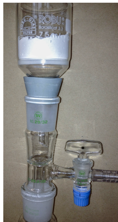
Figure S2. optimized arrangement for filtration over Celite.
